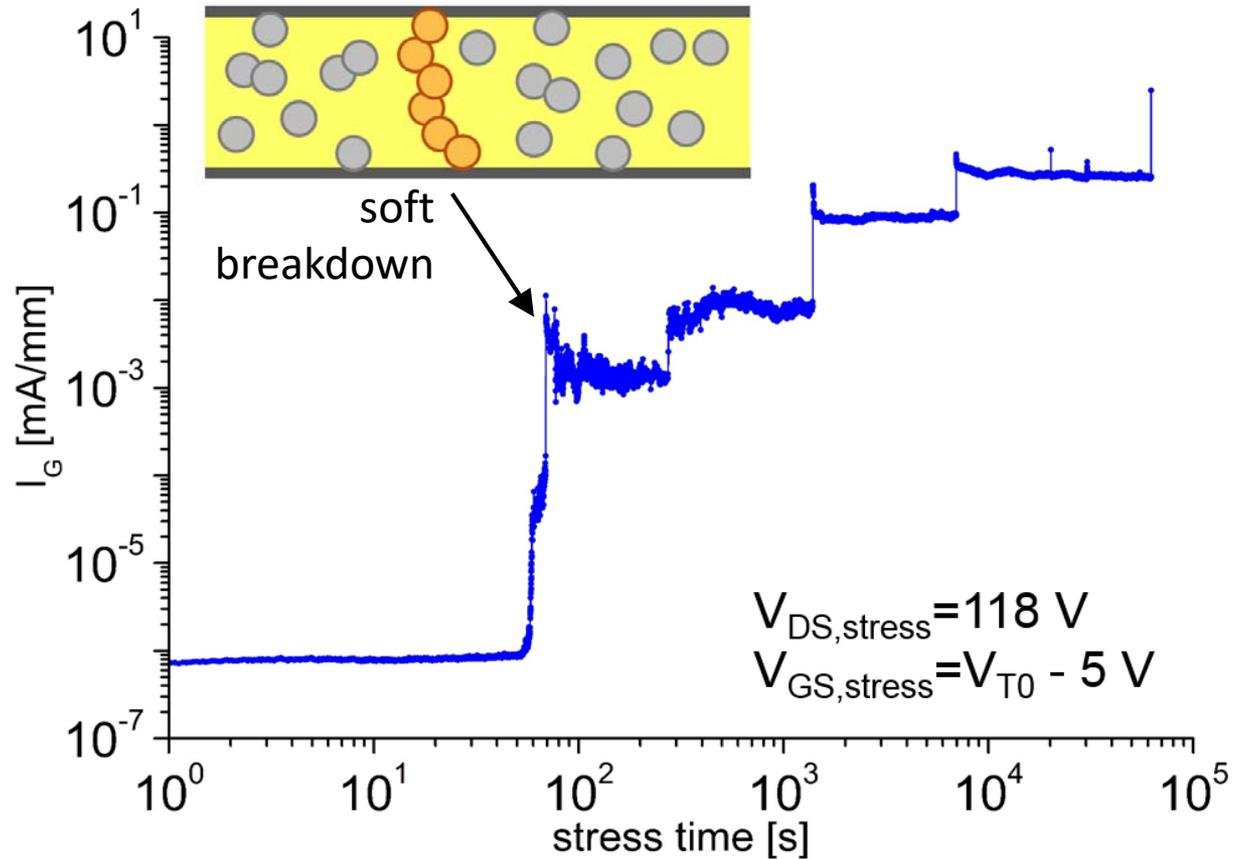
$I_G = I_D \rightarrow$  damage at drain-side edge of gate
